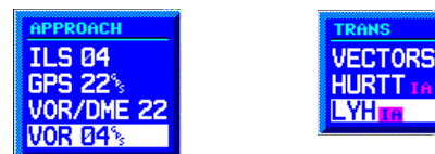
Figure 6-11 Approach and Transitions Windows
